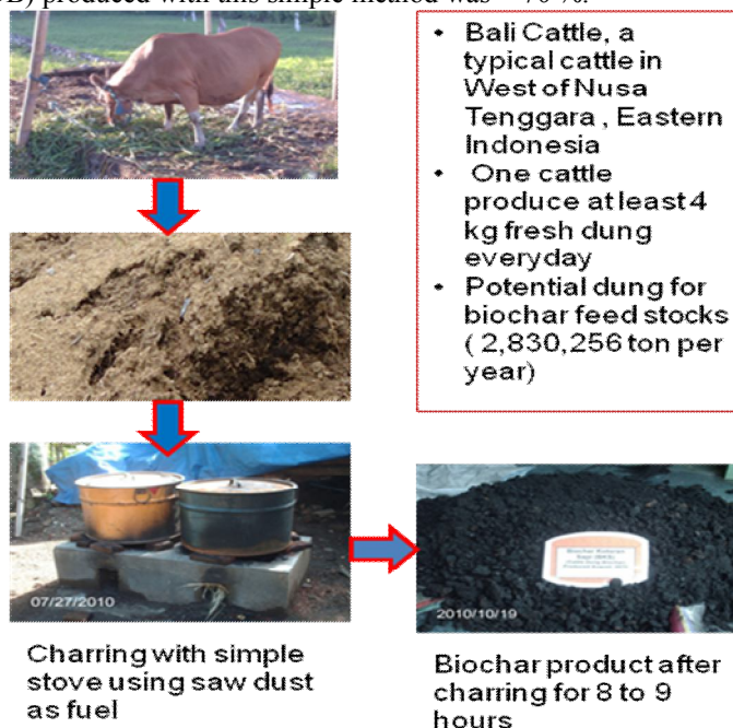
Figure 1. Simple biochar production made from Cattle Dung
