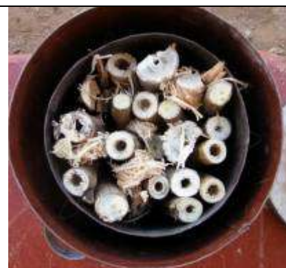
A Champion reactor made in Uganda, partially loaded with vertically placed bamboo sticks (Photo: Christoph Messinger)
