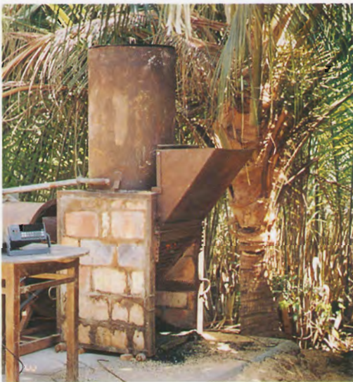
Figure 3. Inclined grate furnace with cyclonic ash separator.
